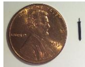
Figure 2. The microdevice located to the right of a penny has 18 reservoirs used to dispense drugs.
